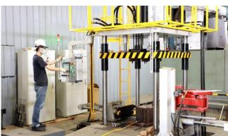
Construction of the first domestic low-pressure casting foam forming manufacturing equipment for recycled aluminum
